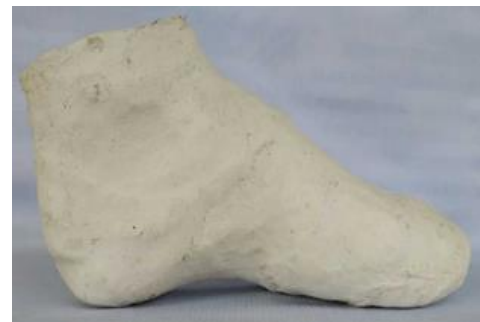
Fig. 2.3: Prepared mold for last making
