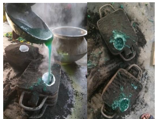
Fig. 2.4: Pouring molten plastic into the mold
