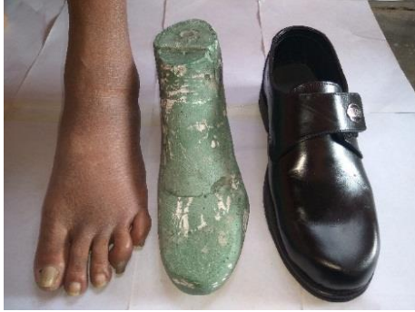
Fig. 2.5: Developed customized last and shoe
